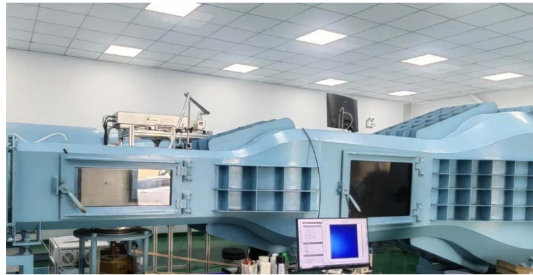
Fig. 1. ZJNU CE TR-PIV system, integrated with the wind-tunnel
